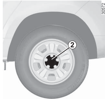
Central wheel trim with visible wheel bolts (example: wheel trim 2)
